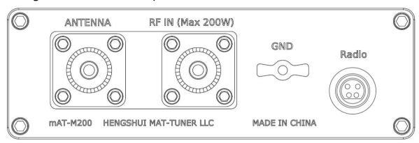
**GND**: Connected to antenna system ground. Correct and good ground wire can ensure the safe operation of the tuner.
